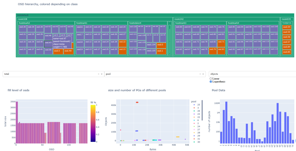
Figure 5.4.: Initial Dashboard showing the relationship between OSDs, PGs and pools
