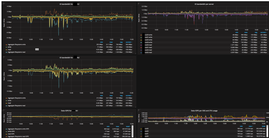
Figure 4.4.: Part of the Grafana Dashboard showing various IO-bandwidth and Data IOPS metrics
